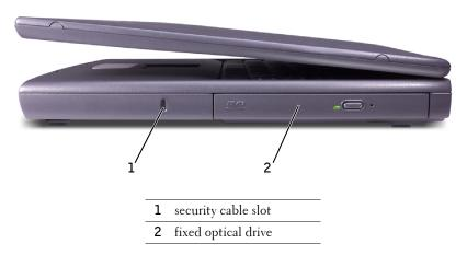
**SECURITY CABLE SLOT** — Lets you attach a commercially available antitheft device to the computer. For more information, see the instructions included with the device.
